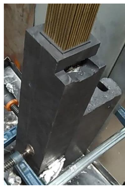
Fig. 1. Final-geometry vessel with metal rods assembled
