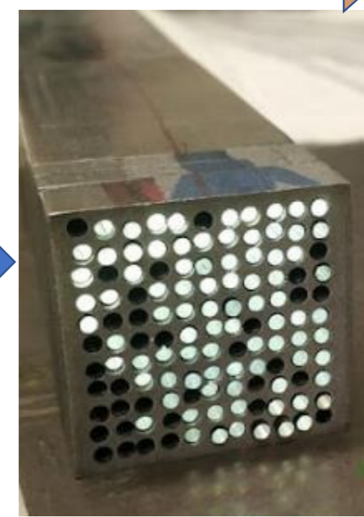
Fig. 3. Absorber with scintillators filled in underway
