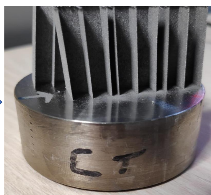
Fig. 5. Testing the incline stability with respect to different angles (0-6°)
